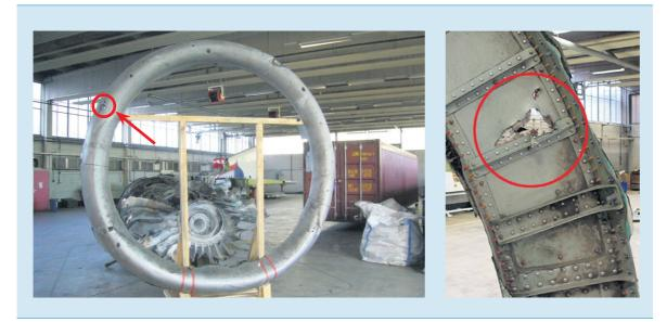
Figure 17: Damaged left engine intake ring, with impact marks seen from the front side (left photo) and from the rear side (right photo). (Source: Dutch Safety Board)
