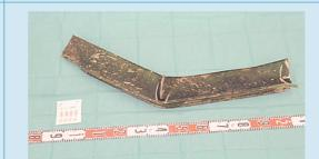
Part of stabilizing fin during identification at Gilze-Rijen Air Force Base. (Source: Dutch Safety Board/Dutch National Police)
