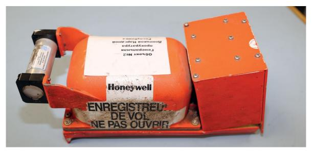
Figure 8: Cockpit Voice Recorder. (Source: Dutch Safety Board)
